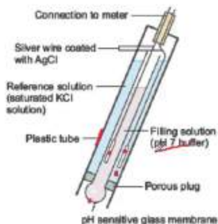
Figure 3.4.2.1: Working of pH Electrode probe [131]
